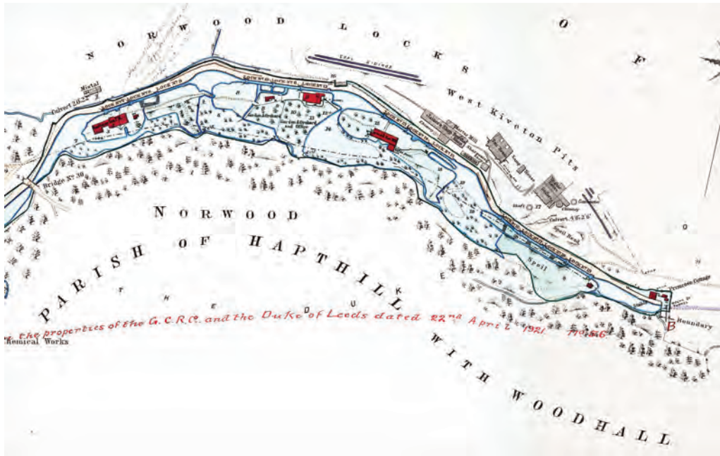
The Norwood flight of three triple and one quadruple staircase locks leading up to the Western portal of Norwood Tunnel. Railway map dated 1892
